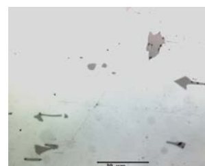
Extremely hard titanium carbides inserted into the steel.
