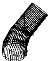
ELBOW Tapered lobster back development.
