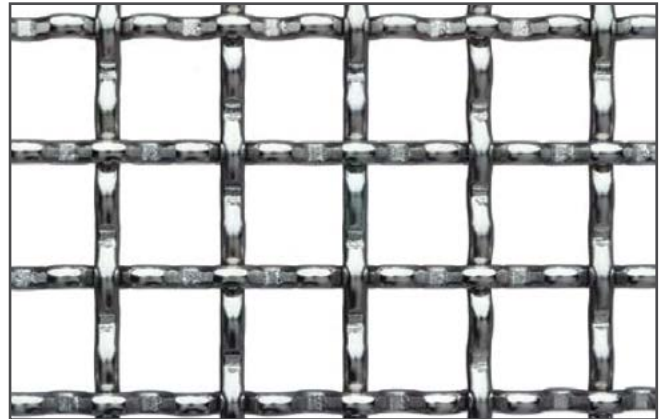
12.7mm Aperture x 3.0mm Wire Dia. / Intercripped
