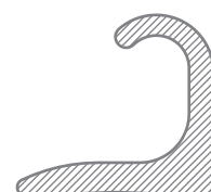
UA1413 24mm x 22mm Heavy Bus Drip Mould 0.431 kg/m
