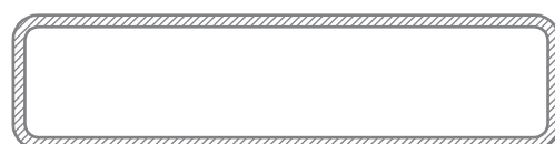
UA6507 65mm x 16mm x 1.4mm Rectangular Hollow 0.576 kg/m
