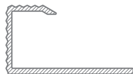
UA4414 13mm Serrated Capping 0.224 kg/m
