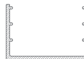
UA2096 38.10mm x 25.40mm Handrail Channel 0.394 kg/m
