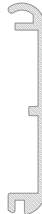
UA2907 90.10mm x 16mm Internal Boat Gunnel 1.107 kg/m
