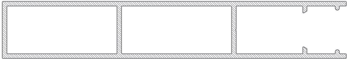
UB025150 25mm x 150mm Batten Outer 2.009 kg/m
