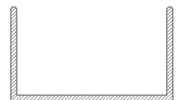
UA6907 40mm Coolroom Channel 0.391 kg/m
