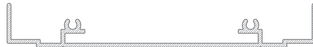
UA8864 133.20mm x 19mm Sign Box Frame 0.986 kg/m
